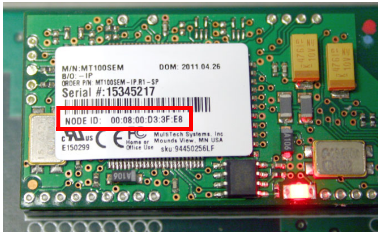
Figure 5-36 Locating the NODE ID (MAC address) on the ethernet modem
