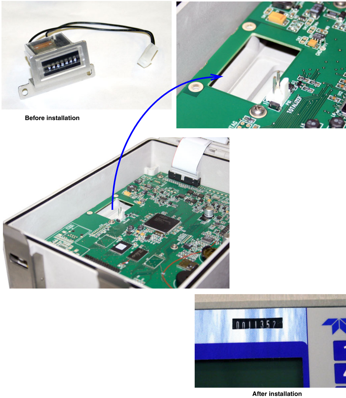
Figure 5-11 Optional non-resettable totalizer installation
