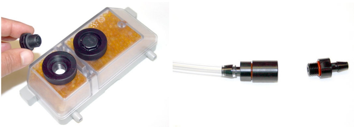
Figure 5-30 Reference port kit: Remove filter and barb
